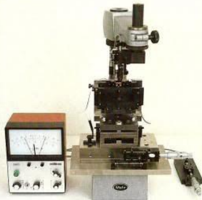
Fig. 25 With this slant measurement tool – BASF's own unique construction, as is the mechanical reference cassette – the accuracy of the pins and stays is measured.
